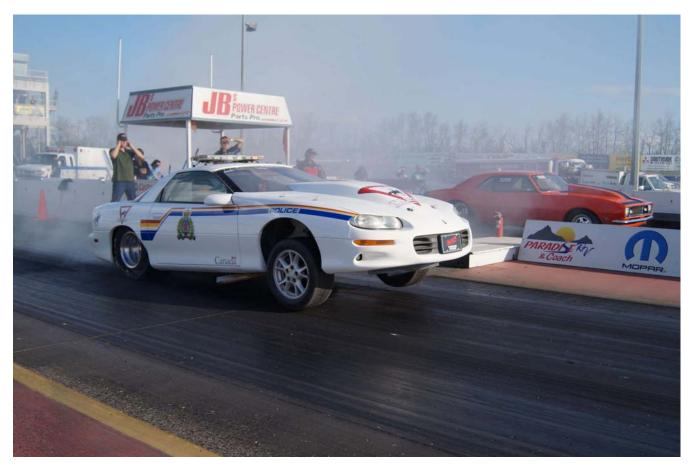
Equipped with a 454 Chevy engine bored and stroked to 489, the Camaro will run 11.2 seconds in the quarter mile at 198 km/h.
